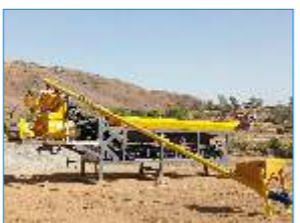
Mobile Batching Plant
