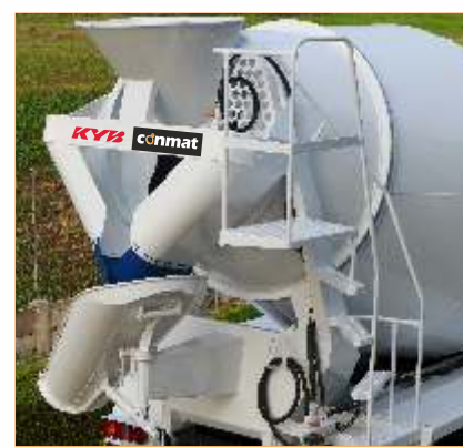
Staircase to inspection platform is designed for operator comfort without compromising safety
