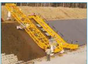
Concrete Canal Paver
