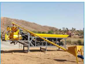
Mobile Batching Plant
