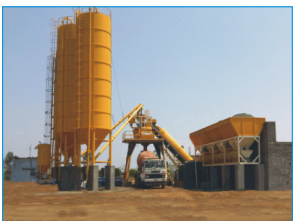
Concrete Batching Plant
