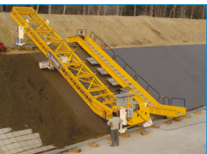
Concrete Canal Paver
