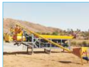
Mobile Batching Plant
